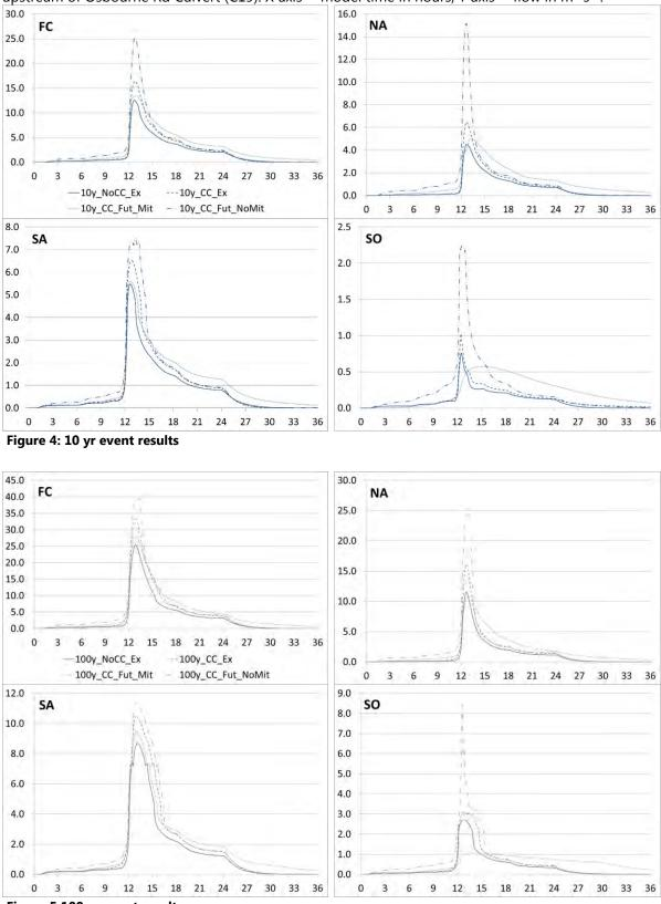
FC = Full catchment (C2), NA = Northern Arm (C1), SA = Southern Arm (C6) SO = Southern Arm upstream of Osbourne Rd Culvert (C19). X axis = model time in hours, Y axis = flow in  $m^3 s^{-1}$ .
