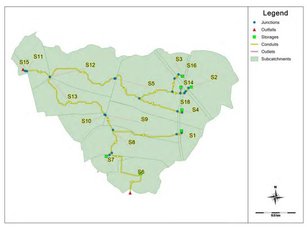
Figure 1 PC SWMM model catchments
