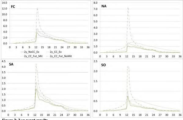
C = Full catchment (C2), NA = Northern Arm (C1), SA = Southern Arm (C6) SO = Southern Arm upstream of Osbourne Rd Culvert (C19). X axis = model time in hours, Y axis = flow in  $m^3 s^{-1}$ .
