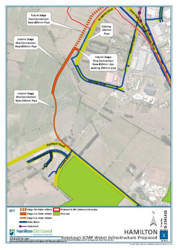
Figure 3-19: Water infrastructure staged construction
