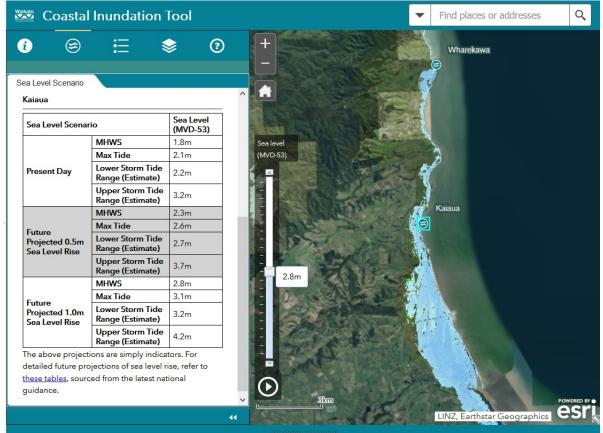
Figure 60 The Wharekawa coast showing the degree of coastal inundation in 2120 when mean sea level is predicted to reach 2.8 m (MVD-53) (actually 2.9 m (RCP8.5), but the Coastal Inundation Tool is in 0.2 m increments)
