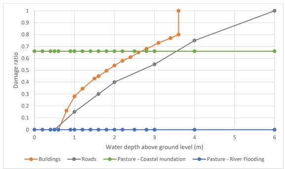
Figure 14 Fragility functions used to estimate losses (damage ratio) in this quantitative risk assessment (note: buildings function has been moved along the x-axis by 0.6 m to account for building floor levels – see below)
