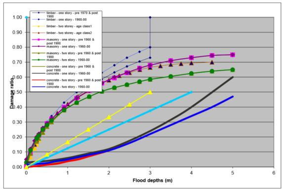
Figure 16 Flood fragility curves for various building types, with flood depth being depth above floor level (Reese & Ramsay, 2010)
