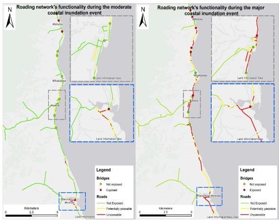
Figure 43 Exposure of roads and bridges to coastal inundation (note: potentially passable is <0.5 m flood depth; unpassable is >0.5 m flood depth)
