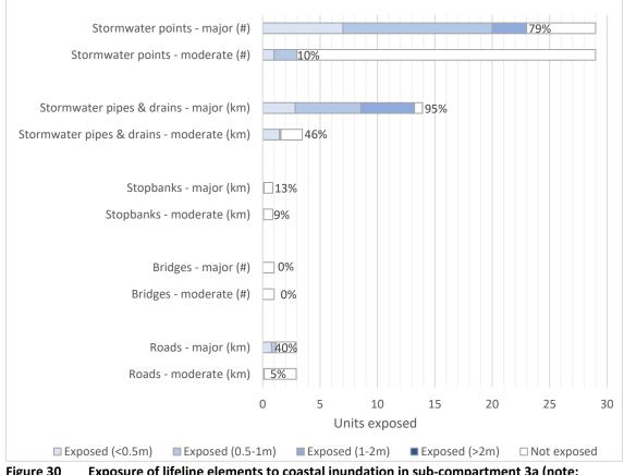
Figure 30 Exposure of lifeline elements to coastal inundation in sub-compartment 3a (note: percentages refer to total % exposed)
