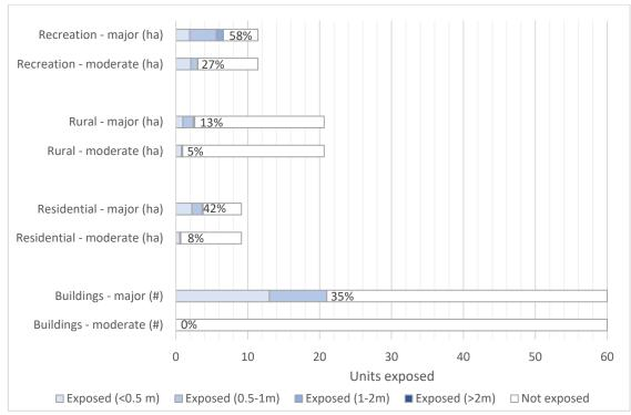
Figure 34 Exposure of buildings and land use types to coastal inundation in sub-compartment 5a (note: percentages refer to total % exposed)
