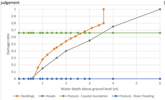
displacement days (as a function of damage ratio). A range of fragility functions have been considered for each element and the most appropriate function selected based on expert judgement (
