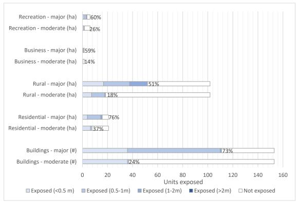
Figure 26 Exposure of buildings and land use types to coastal inundation in sub-compartment 2a (note: percentages refer to total % exposed)
