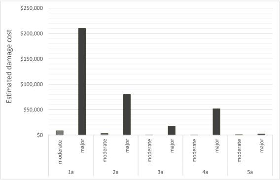
Figure 55 Estimated cost of damage to roads from coastal inundation by sub-compartment, where sub-compartment names are: 1a Pūkorokoro Miranda; 2a Kaiaua township; 3a Whakatiwai; 4a Waihihi; 5a Waharau
