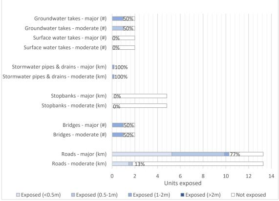
Figure 23 Exposure of lifeline elements to coastal inundation in sub-compartment 1a (note: percentages refer to total % exposed)
