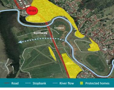
The spillway diverts large volumes of flood water while providing the level of protection required for Thames, especially as the Kauaeranga River responds quickly to rain.
