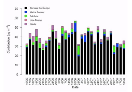
Figure 1.6 Barplot of source contributions on days (during 2014) when PM<sub>10</sub> concentrations exceeded the Ministry for the Environment "Alert" level (33 µg m<sup>3</sup>).
