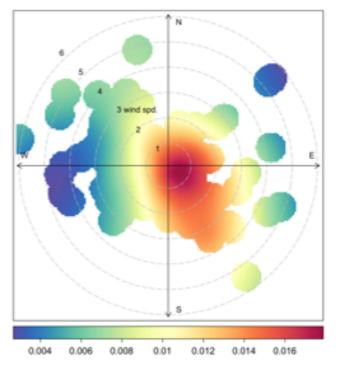
Figure 1.5 Polar plot of secondary sulphate contributions. The radial dimensions indicate the wind speed in 1 m s<sup>-1</sup> increments and the color contours indicate the average contribution to each wind direction/speed bin. The legend below the plot provides an indication of the concentration combined with the frequency of occurrence. The warmer <u>colours</u> indicate higher concentrations and frequencies.
