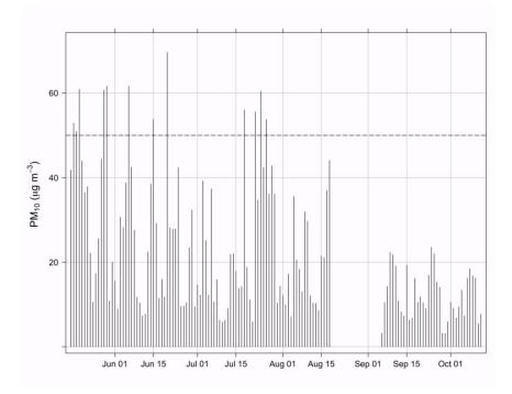
Figure 2-1: Time-series of PM  $_{10}$  concentrations in 2014. The hashed line indicates the NESAQ (50  $\mu g$  m  $^{-3}$ ).
