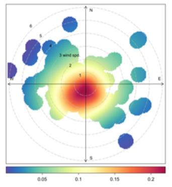
Figure 1.4 Polar plot of biomass combustion contributions. The radial dimensions indicate the wind speed in 1 m s<sup>-1</sup> increments and the color contours indicate the average contribution to each wind direction/speed bin. The legend below the plot provides an indication of the concentration combined with the frequency of occurrence. The warmer colours indicate higher concentrations and frequencies.
