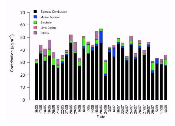
Figure 6-1: Barplot of source contributions on days (during 2014) when PM<sub>10</sub> concentrations exceeded the Ministry for the Environment "Alert" level (33 μg m<sup>-3</sup>).
