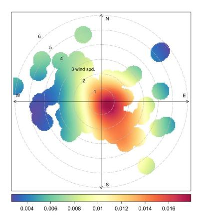
Figure 5-2: Polar plot of secondary sulphate contributions. The radial dimensions indicate the wind speed in 1 m s<sup>-1</sup> increments and the color contours indicate the average contribution to each wind direction/speed bin. The legend below the plot provides an indication of the concentration combined with the frequency of occurrence. The warmer colours indicate higher concentrations and frequencies.
