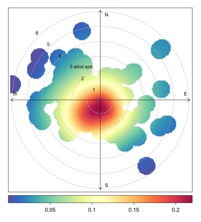
Figure 5-1: Polar plot of biomass combustion contributions. The radial dimensions indicate the wind speed in 1 m s<sup>-1</sup> increments and the color contours indicate the average contribution to each wind direction/speed bin. The legend below the plot provides an indication of the concentration combined with the frequency of occurrence. The warmer colours indicate higher concentrations and frequencies.
