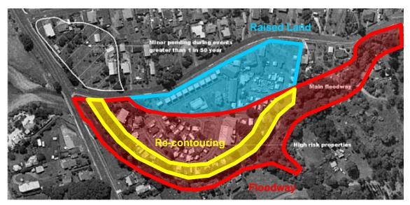
Figure 10 Proposed floodway works
