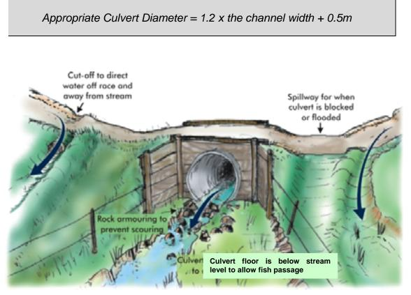
Figure 5 Outlet of typical Best Practice single barrel circular culvert
