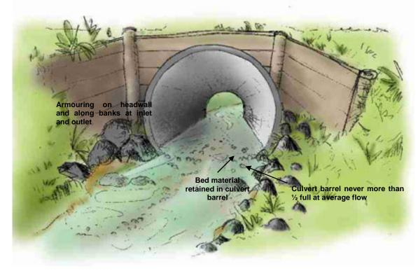
Figure 6 Typical Best Practice single barrel circular culvert
