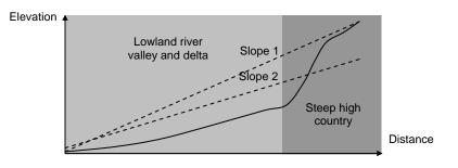
Figure 14 Typical profile of a river
