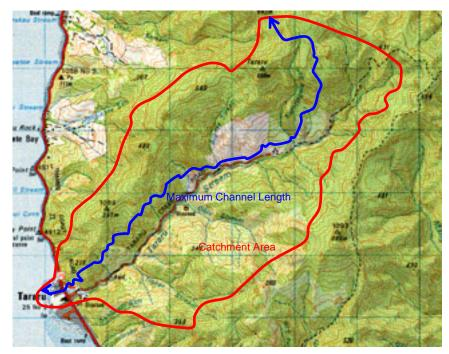
Figure 13 Characteristics of a catchment
