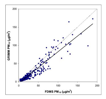
Figure 2-2 Scatterplot of hourly average  $PM_{10}$  data obtained from an FDMS permanently installed at Woolston, Christchurch, and a GRIMM instrument, collocated between 6 August and 20 August 2008 (from Olivares et al. 2008b). Linear regression line (solid line) has equation y=0.9x-4 ( $r^2=0.89$ ) and 1-1 line is plotted for comparison (dotted line). FDMS data were provided by Environment Canterbury.
