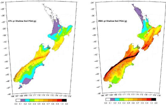
Figure 9 : 2010 National seismic hazard model for New Zealand showing expected PGA's for a 475 and 2,500 year return period earthquake for shallow soils (Saunders & Berryman 2012)
