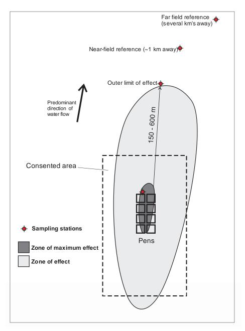
Figure 6. Schematic showing the application of seabed effects zones to aquaculture, with compliance at zone boundaries regulated by environmental quality standards and sampling at set stations with varying proximity to pen structures.
