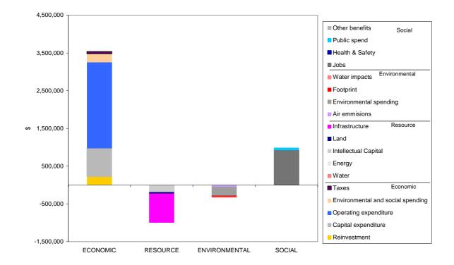
Fig. 3 Sustainability profile for Disposal scenario 2—disposal to landfill with waste diversion.
