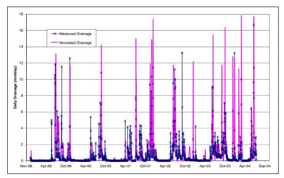
Figure 7: Simulated subsurface drainage compared to the measured data (on an event basis for the Howie artificial drainage system)
