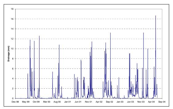
Figure 4: Measured artificial drainage flow from Toenepi from Dec 1998 to Jun 2004
