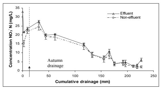
*Figure 3: Trend in nitrate-N concentrations with accumulated drainage (Houlbrooke et al, 2003)*
