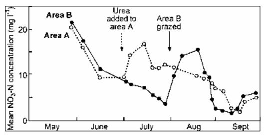
Figure 1: Nitrate-N concentrations in tile drainage discharging from two areas, with either urea fertiliser or grazing treatments (Monaghan et al. 2002)
