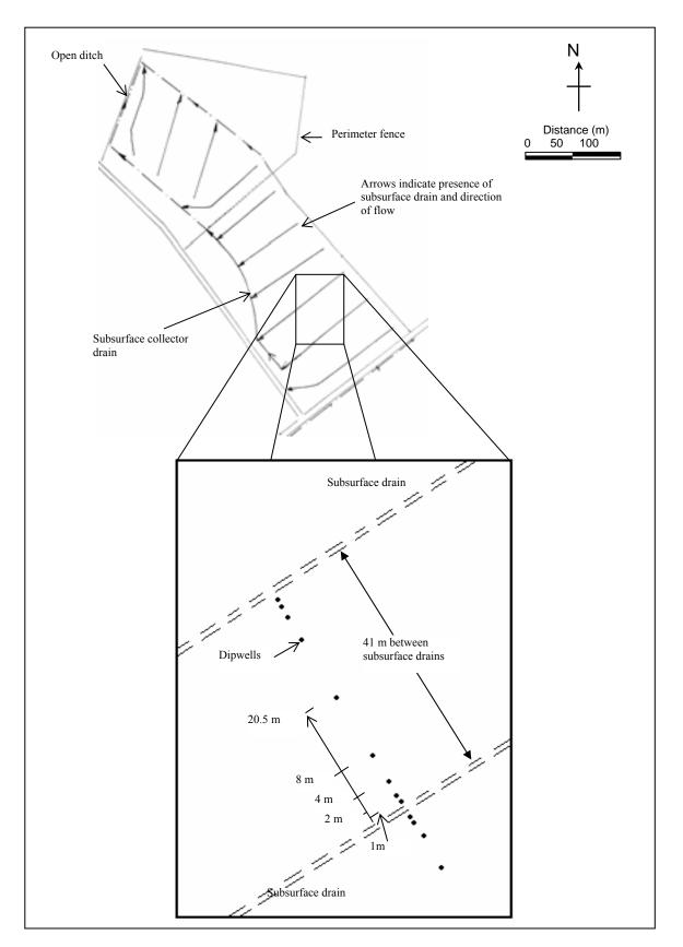
Layout of subsurface drainage, collector drains and open ditch (Stafford, 2002).
