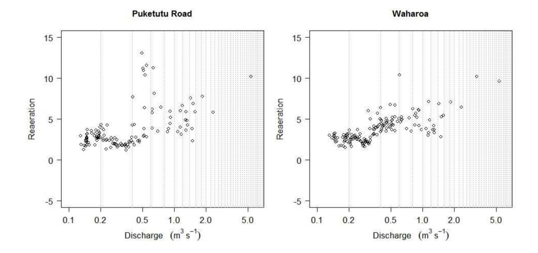
Figure 3-20: Scatter plots of the estimated reaeration coefficient (k<sub>2</sub>) and river flow at the Puketutu Road and Waharoa sampling sites on the Waitoa River.
