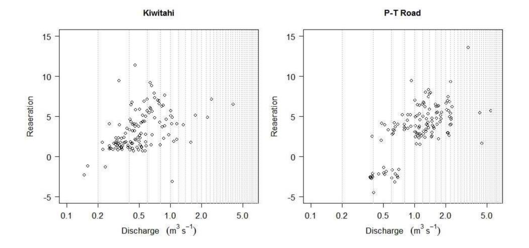
Figure 3-19: Scatter plots of the estimated reaeration coefficient (k<sub>2</sub>) and river flow at the Kiwitahi and Paeroa-Tahuna Road sampling sites on the Piako River.
