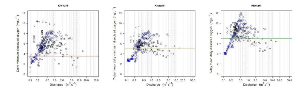
**Figure 3-14:** Scatter plots of daily minimum, 7-day mean daily minimum and 7-day mean daily dissolved oxygen concentrations against mean daily flow. Data are for the Piako at Kiwitahi. Circles represent data from 2011-12 and crosses 2012-13 sampling periods. Note that the x-axis is a logarithmic scale. The recommended imperative ecosystem protection levels for each dissolved oxygen statistic are shown as solid horizontal lines.
