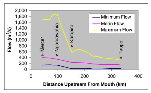
Figure 3: Maximum Minimum and Mean flows versus Distance Upstream of the Mouth
