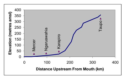
Figure 1: Waikato River - Profile of Water Surface Elevation
